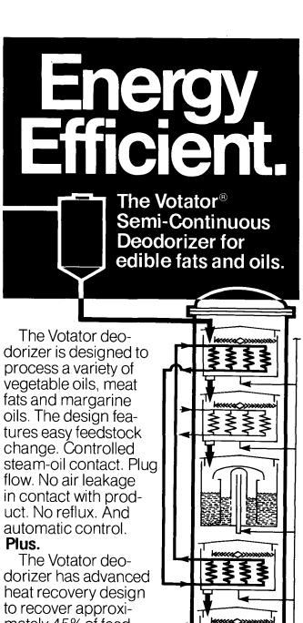
The Votator deodorizer has advanced heat recovery design to recover approximately 45% of feedstock heating requirements. Flexible deodorizing conditions. And increased by-product value.
